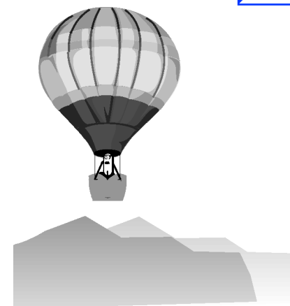
Figure 17.14: A balloon uses the buoyancy of hot air to lift off.
