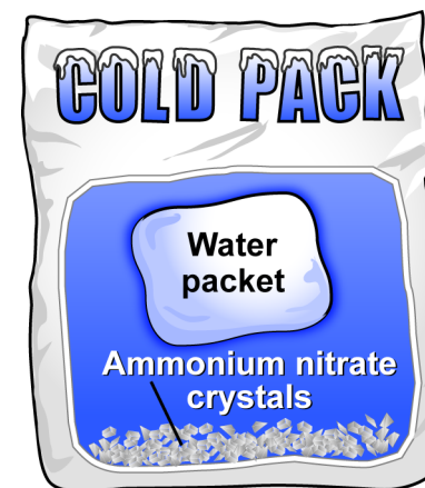
Figure 21.7: An instant cold pack contains ammonium nitrate crystals and a packet of water. When squeezed, the water is released and the reaction occurs.
