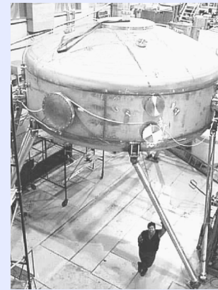
The LDX experiment at MIT uses a superconducting coil to explore fusion energy.
